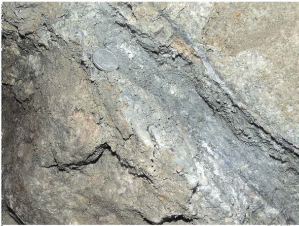
照片 2 马厂箐矿区斑状花岗岩内的脉状辉钼矿化 Photo 2 Veinlike molybdenite mineralization in porphyritic granite from Machangqing ore district
